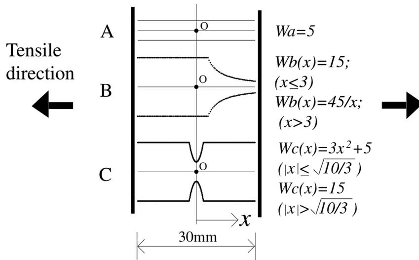
Fig. 4 Shapes of the specimens used for the non-uniform strain field
